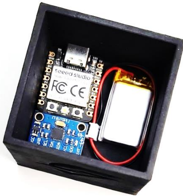
Figure-10 ESP32, MPU6050 Sensor, and Battery Integrated to AkSat U2
